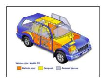
VIP vehicle can be ordered armoured to levels B6 or B7. Most Luxury vehicles are capable of being armoured. Land Cruiser Pick-ups and similar vehicles can also be armoured to protect workers in dangerous areas.
