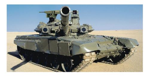
The WASP is state of the art technology for Remotely Controlled Weapon Mounting Systems. It adds significant protection for both the operator and the vehicle that it is mounted on. Controlled from within the vehicle the Operator can scan for ground or air threats and protect for 360 degrees around the vehicle.
